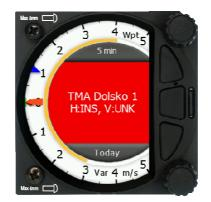
The first row is a name of the airspace. You can terminate a warning for 5 minutes by pressing an upper button or lower button, which will cancel it for today.
