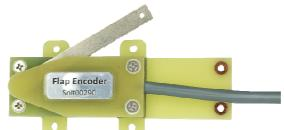
The Flap sensor must be connected to the CAN bus through a CAN bus (Y) splitter. Any remaining ports on the Y CAN splitter must be terminated with a CAN terminator.
