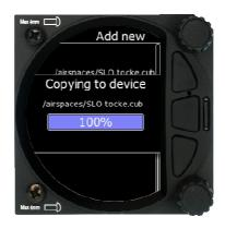
The LXNAV ASAPT database file format is also supported and can be loaded into the system.
