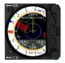
The first page shows a line to a selected waypoint, the name of the selected waypoint at the top of the screen and the relative bearing with chevrons indicating the direction to turn towards the selected waypoint.
