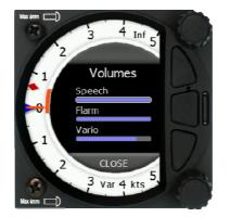
The lower rotary knob is used to adjust settings within the current mode or within menus. With the lower rotary push button, it is possible to toggle between the MC and the Ballast and Bugs settings. In all other menus this knob is used for setting values and editing texts.
