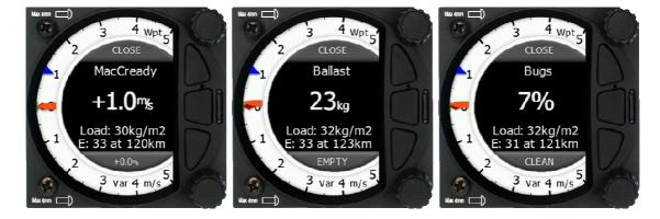
To change the McCready value, press the bottom rotary knob and press on MC/BAL. A short press of the lower rotary knob moves from McCready to the Ballast box and pressing the lower rotary knob again will open the Bugs box. If no action is performed within 3 seconds, the box will close, or you can also press CLOSE anytime (lower push button).
