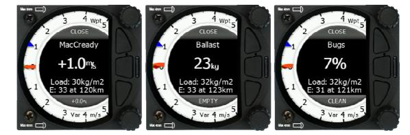
Rotate the lower knob to modify any setting. Next check the safety altitude (height above destination, arrival altitude) setting.
