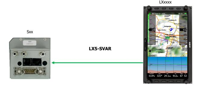
This configuration is used for example when using your Sxx vario together with Oudie and LXxxxx. **LX5-SVAR** is connected to **GPS port** and **CC-NP-OUDIE** cable to **PDA port**.
