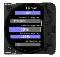
With a push of the lower rotary button you can activate the slide control and then by rotating the knob you can select the preferred value and confirm it via the push button.
