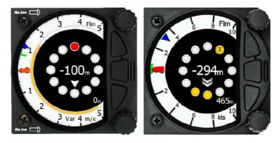
The warnings continue as long as FLARM calculates a threat of collision. The warning level may decline or be cancelled, depending upon the prediction. The warnings are selective; they are only issued if the calculation reveals a high probability of collision in the near future.
