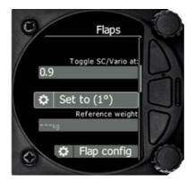
When all flap positions are set, a green dot will be displayed with current flap position. If flap labels are not set yet, press **EDIT** to name the labels. Flap labels must be entered with increasing speed range. It is recommended that flaps labels are set together with the speed range in the Polar and Glider setup. It is also possible to toggle between cruise and climb mode using the flap sensor.
